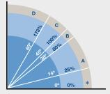
**D**: Every tile should be securely fastened (Nailed, screwed, clipped...) (60° / 203/4:12).
